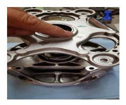
5)\* Set up the flyweights as described in this instruction manual for your desired application See the proper "Set-Up Guide" for your vehicle (for versions other than PRO XP see back section). Take note of your set up guide and set up the flyweights, then install the flyweights into the drive clutch. Use Blue Loctite on the flyweight pivot bolt nuts. Be sure to read the complete document before continuing.
