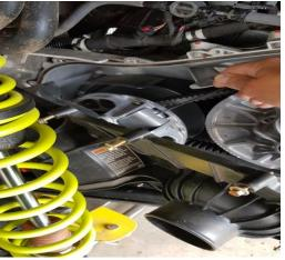
3) Adjusting the tip weight (cross hole at the tip of the flyweight)
