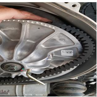
the tool into the threaded hole in the secondary clutch. This will spread the sheaves apart to allow easy
