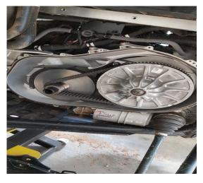
Remove the 6 bolts and clutch cover plate. Be sure to look for alignment marks on cover plate (X on the cover and spider), or mark the clutch with a magic marker for orientation during re-installation. Be careful when removing cover plate bolts, the primary spring is under pressure.
